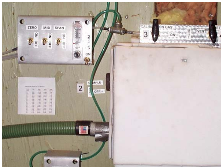
FIGURE 4B. Photo of VOC sampling system showing heated sample box (with white insulation), toggle valves and flow meter for calibration gases (upper left), on/off valve for calibration gas (3 at upper center right), heated sample line to analyzer (green tube, lower left), valve for sample (2 at center), toggle valve to vacuum pump (near calibration gas valves), and vent/flowmeter valve (4 at upper right).
